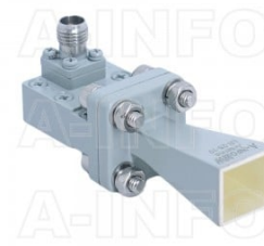
LB-28-10-C-KF Standard Gain Horn Antenna 26.5-40GHz 10dB Gain 2.92mm Female
